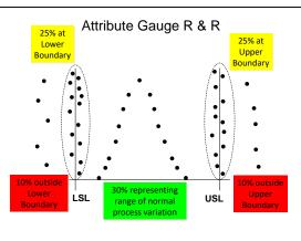
Depending on the characteristic, the above parts should be independently measured with a variable gauge (such as a CMM or other known standard) so that the physical measurement of each part is known.
